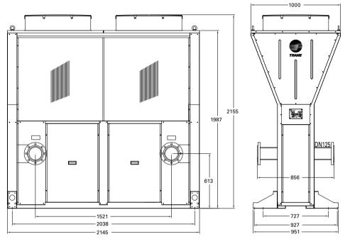
Outlet pipe is at near control box side, and inlet pipe is at far side of control box.
