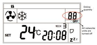
Notes: A. If the online quantity displayed is inconsistent with the actual quantity, inspect whether the connecting line is connected correctly, or confirm whether the unit dial code is correct.
