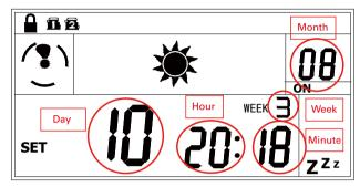
Note: after the master controller is installed for the first time or the battery is replaced, the clock must be adjusted; otherwise, the clock will not work, and the balance running time will be invalid.
