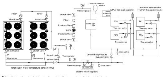
Note: 1)Each branch needs to install a water flow switch, which is connected to the A0 host chiller in series.
