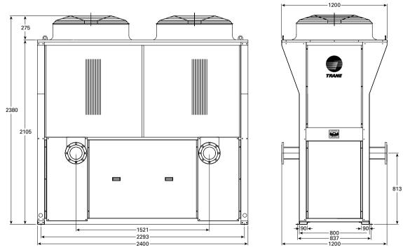
When facing to the electric cabinet. The left water pipe is outlet pipe, and the right water pipe is inlet pipe.
