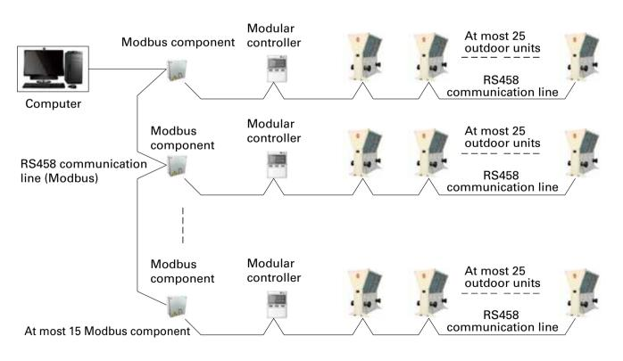
For the specific wiring and operation of Modbus components, see Operation Manual for CXAJ Series Modbus components.
