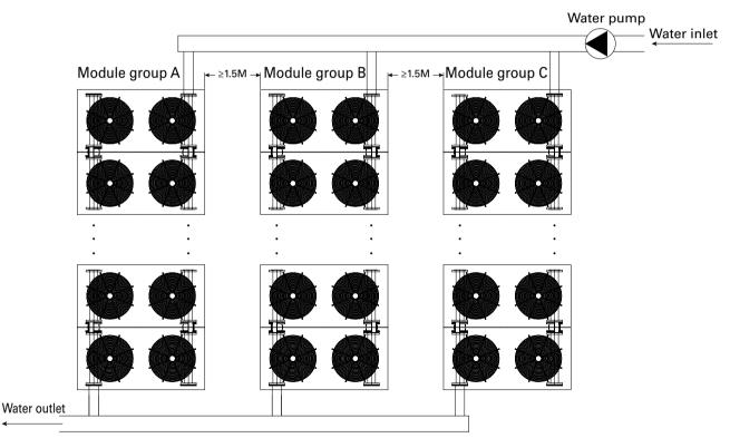
Note: CXAJ/CGAJ065 multi-module combination includes at most 8 sets per group, CXAJ/CGAJ130multi-module combination includes at most 4 sets per group, and no direct return connection is allowed.
